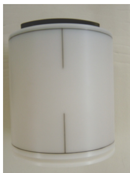
Fig. 4. PET source consists of a solid radioactive cylinder phantom.
