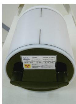
Fig. 4. PET source consists of a solid radioactive cylinder phantom.
