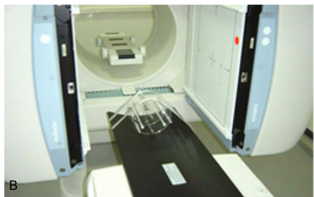
Fig. 1. (A) Line source setup of detector (B) SPECT phantom NEMA tests with scatter
