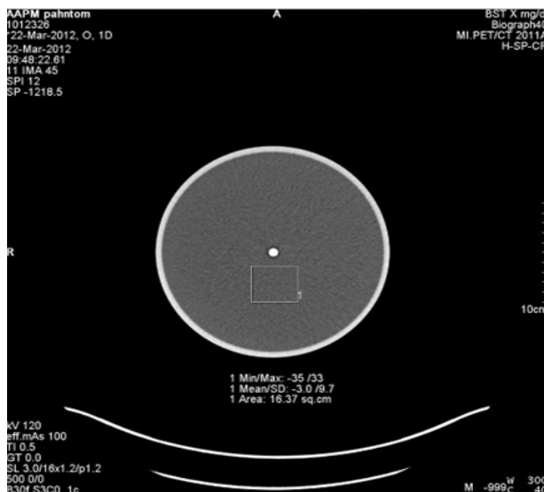
Fig. 5. Drawing ROI for noise test.
