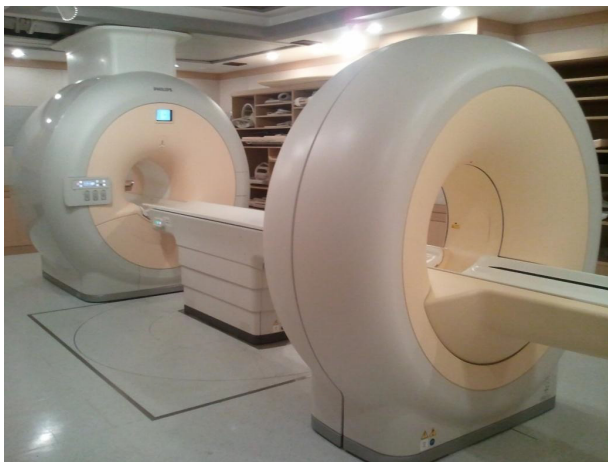
Fig. 1. The Philips Ingenuity PET/MR TF system is a hybrid imaging system with Philips time of flight GEMINI TF PET and Achieva 3T X-series MR system. A turntable patient handling system facilitates patient motion between the MR system on the left and the PET system on the right.
