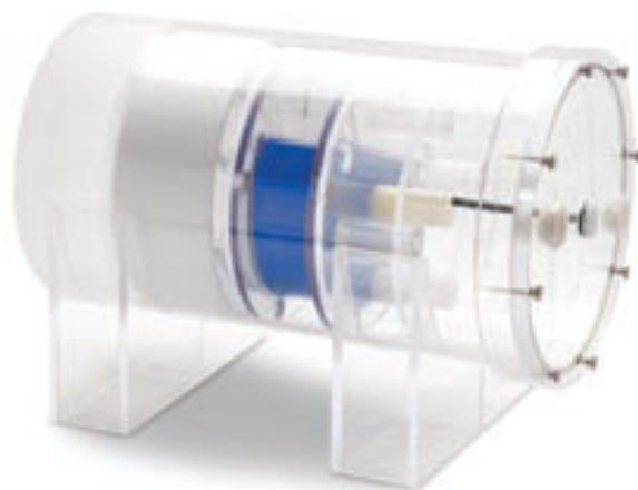
Fig. 1. AAPM CT Performance Phantom was used to evaluate the noise and spatial resolution of CT study.
