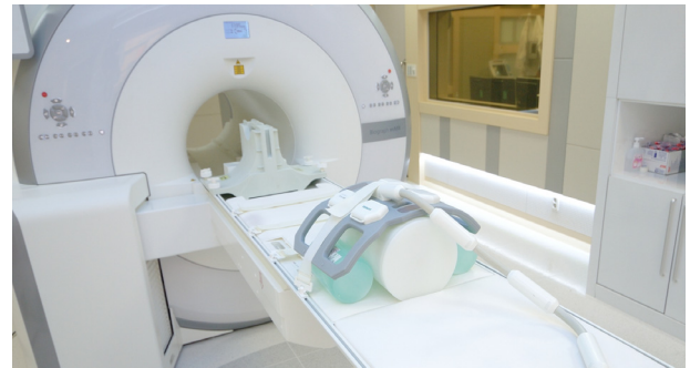
Fig. 8. Cylindrical uniformity phantom is on the spinal coil, surface coil with 2 MRI phantom at both sides.
