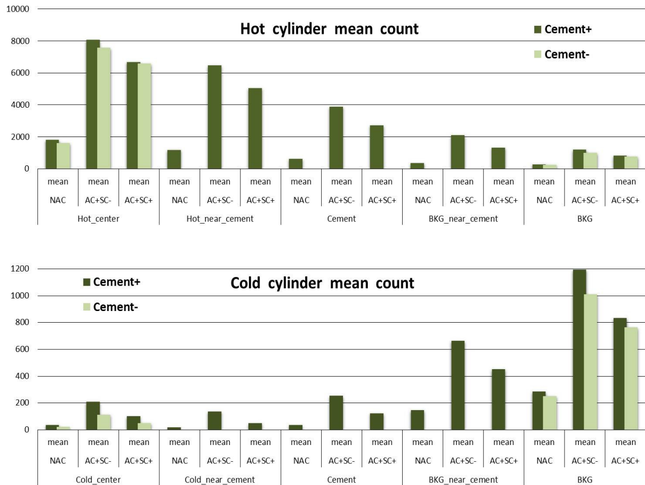
Fig. 10. As the graph showing the change of the mean count on the 5 types of detail regions centering the cylinder when the bone cement exists, the mean count of AC+SC- is the highest.
