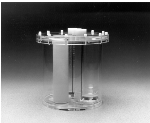
Fig. 1. NEMA-1994 Phantom was used to evaluate the mean count of SPECT/CT study.
