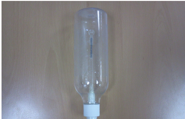
Fig. 2. A customized thyroid-mimicking phantom consisting of an acrylic bottle and a hollow sphere was used for this study.
