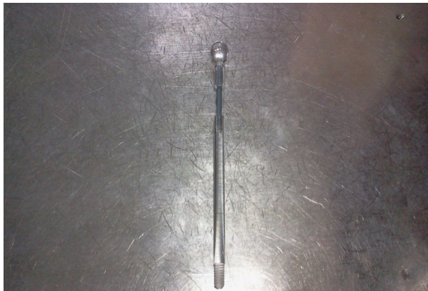
Fig. 1. This is a Hollow sphere which is removable and fillable (Diameter: 9.9 mm, Volume: 0.5 cc).
