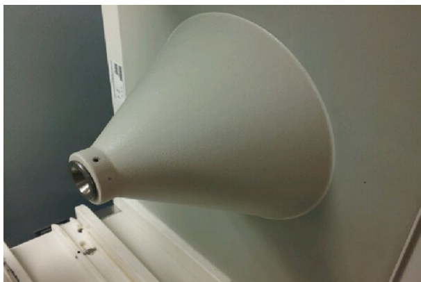
Fig. 2. Pinhole collimator was used for this study.
