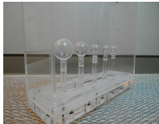
Fig. 2. Self-development Phantom was used to evaluate the CNR and Count rate of BSGI.
