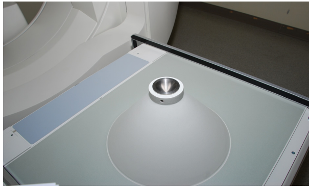
Fig. 1. Pinhole collimator was used conventional system.
