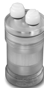
Fig. 4. Micro-PET phantom was used for evaluating cylinder diameter.
