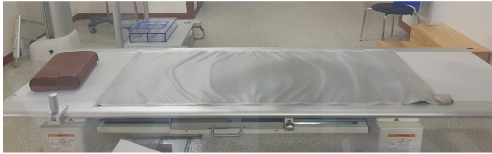
Fig. 4. The figure above is the heating mat made of carbon fiber.
