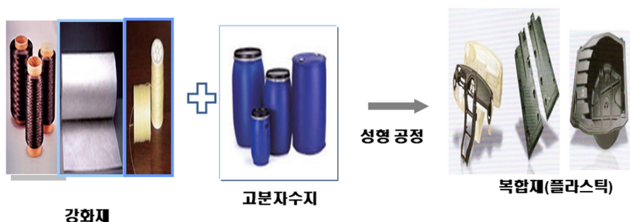
Fig. 2. The figure above shows the process of making carbon composites using reinforcing materials and polymer materials.
