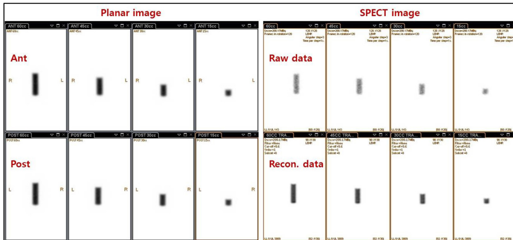
Fig. 6. Planar images(left) and SPECT images(right) were acquired by reducing the volume of the phantom by 25% each.
