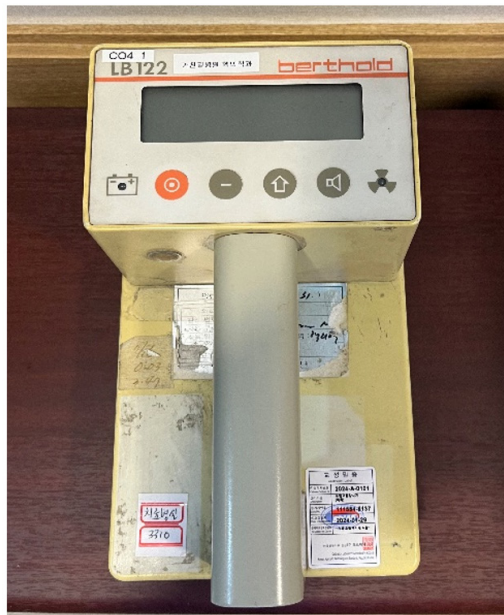
Fig. 1. A surface contamination counter is used to measure the dose of food left behind by patients hospitalized in the therapy isolation rooms.
