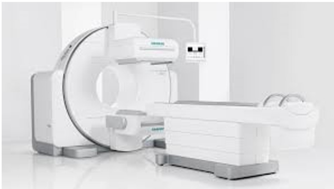
Fig. 1. Dual-head gamma camera was used for image acquisition(Symbia Intevo Bold, Siemens, Germany).
