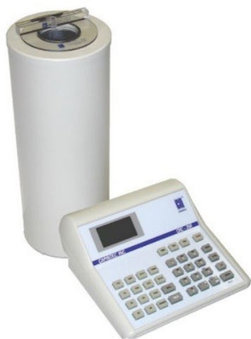
Fig. 2. The CRC-25R radioisotope dose calibrator (A) is employed to accurately measure the activity of various radionuclides, while a Cesium-137 calibration gamma standard source (B), emitting 662 keV gamma rays, is used to verify that the measurement accuracy remains within the specified limits.
