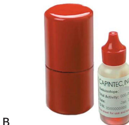
Fig. 2. The CRC-25R radioisotope dose calibrator (A) is employed to accurately measure the activity of various radionuclides, while a Cesium-137 calibration gamma standard source (B), emitting 662 keV gamma rays, is used to verify that the measurement accuracy remains within the specified limits.
