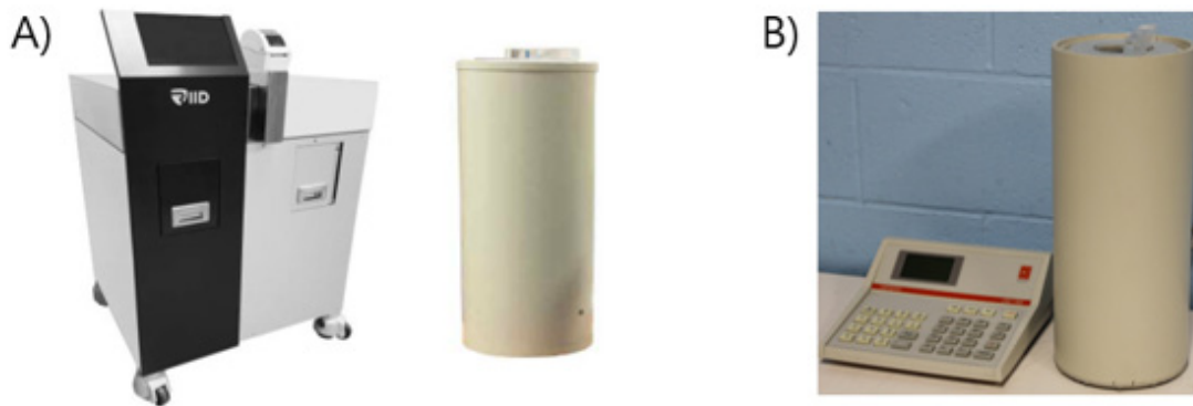
Fig. 2. Photograph of the automated dispensing system and external dose calibrator used in this study. (A) Automated dispensing system RIID (UNITEKO Inc., Korea) with a built-in CRC-PC Smart dose calibrator (Capintec Inc., USA). (B) External CRC-15 PET dose calibrator (Capintec Inc., USA).
