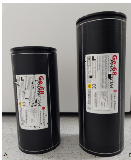
Fig. 2. Ge-68 Annulus phantom used for (a) Discovery MI PET-CT and (b) OMNI Legend PET-CT.
